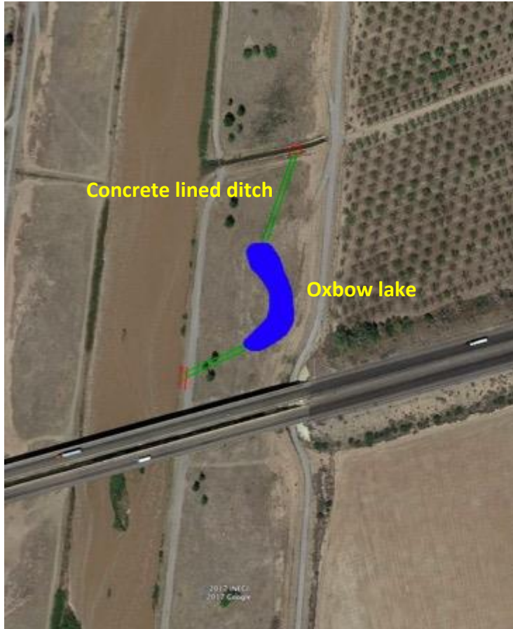
FIGURE 14. Schematic illustration of oxbow lake constructed to provide perennial habitat for native fishes using LCWTF discharge water.
