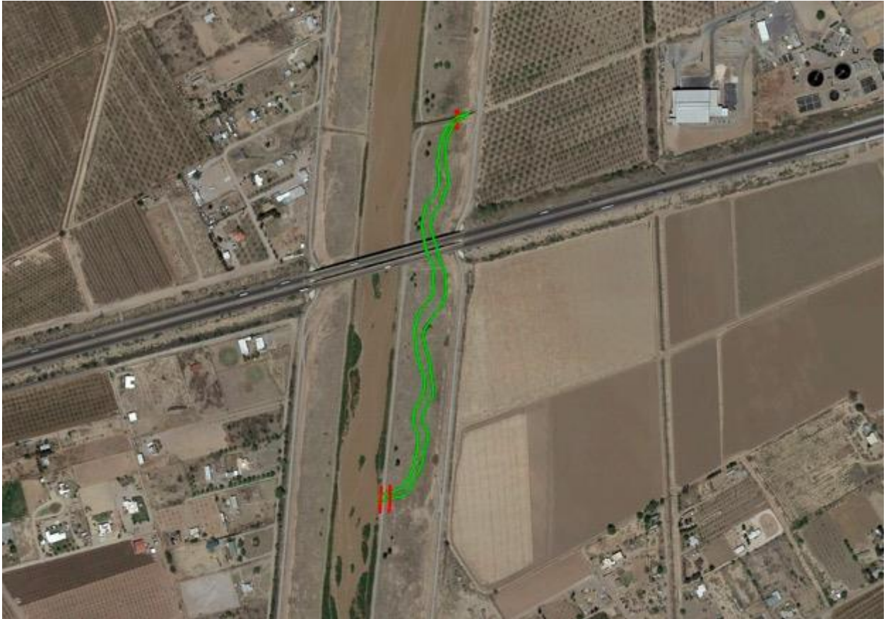
FIGURE 8. Schematic illustration of constructed channel to provide perennial habitat for native fishes using water discharged from the Las Cruces Wastewater Treatment Facility.
