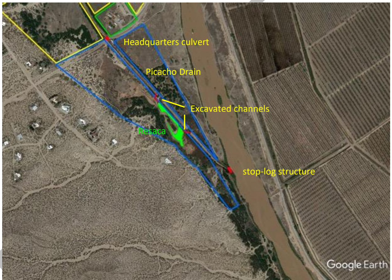
Figure 20. Lower Picacho Drain, headquarters culvert gate, stop-log structure (gated culvert that uses logs or boards to control water passage), Resaca (oxbow lake), and connecting channels.
