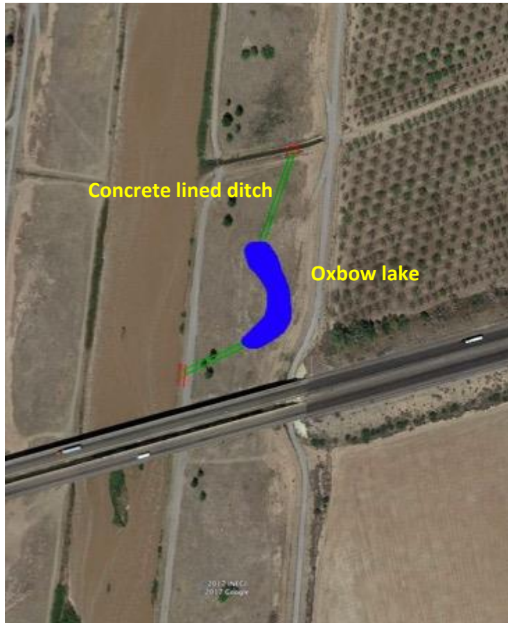
FIGURE 14. Schematic illustration of oxbow lake constructed to provide perennial habitat for native fishes using LCWQTF discharge water.
